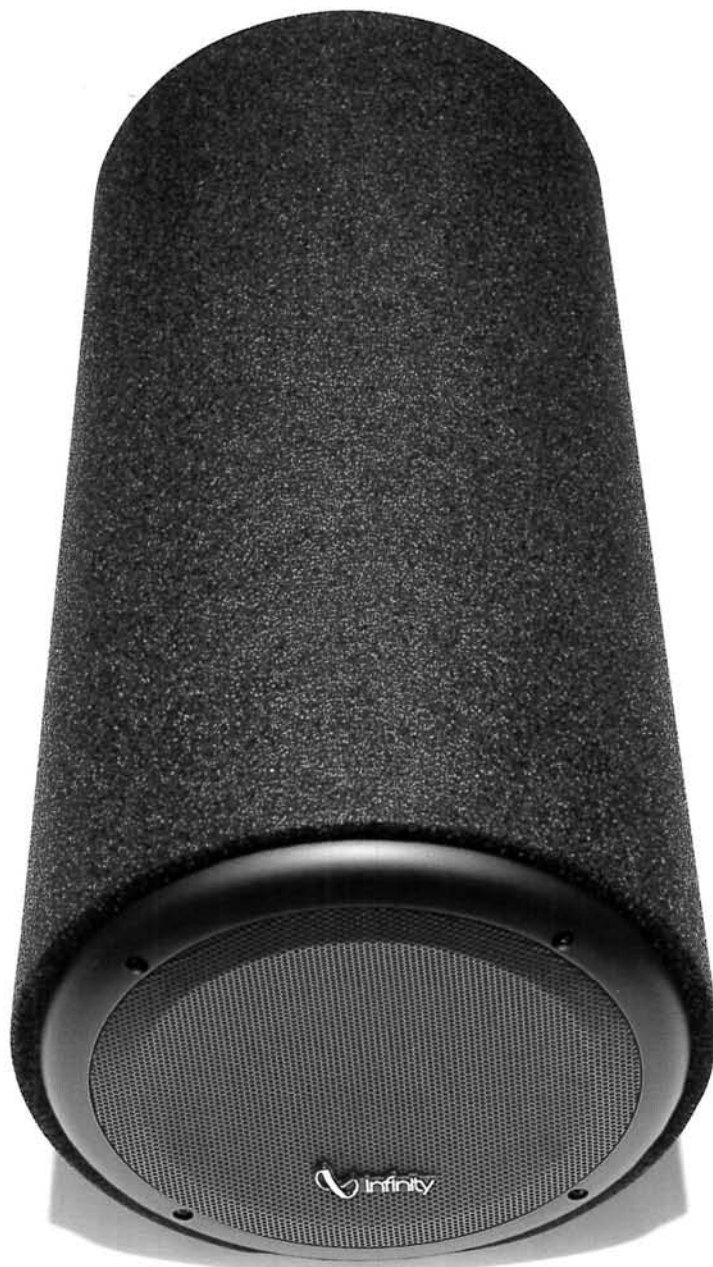
Kappa 120bt Subwoofer Size: 30 cm (12"). Power handling: 250 Watts. Frequency Response: 25-1,000Hz. Sensitivity: 94dB @ 2.83 Volts. Dimensions (Width x Length): 35 x 72 cm
