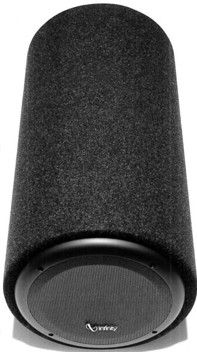
Kappa 100bt Subwoofer Size: 25 cm (10"). Power handling: 200 Watts. Frequency Response: 28-1,000Hz Sensitivity: 93dB @ 2.83 Volts. Dimensions (Width x Length): 31 x 60 cm
